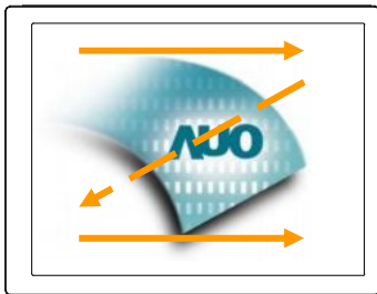
Fig. 1 Normal scan (Pin24, Reverse = Low or NC)
