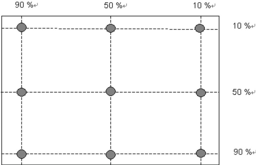
Note 3: The luminance uniformity of 9 points is defined by dividing the minimum luminance values by the maximum test point luminance
