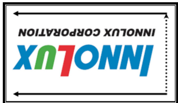
RPFI = high: display with 180degree rotation
