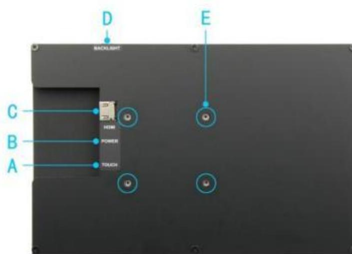
**A: TOUCH touch interface (Micro-USB):** Use Micro-USB cable and signal source device
